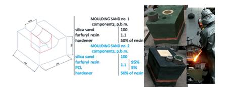
Fig. 2. The scheme of the casting (dimensions in mm), the composition of used sand mixtures, moulds and casting process
