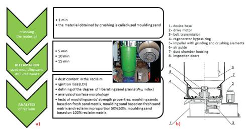
Fig. 3. The schedule of testing moulding sands' ability to mechanical regeneration (a); The RD-6 rotor regenerator: b) fragment of the experimental scheme; c) external view of the regenerator [29,30]
