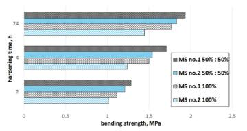
Fig. 8. The influence of PCL additive on bending strength of moulding sand based on fresh silica matrix and the reclaim after 15 min of regeneration
