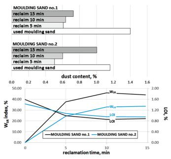
Fig. 4. Dust content, ignition loss (LOI) and the degree of liberating sand grains from binders left-overs ( $W_{SR}$  index) vs regeneration time for used moulding sands (0 min) and reclaimed sands after 5, 10 and 15 min of regeneration
