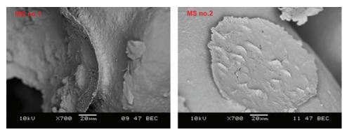
Fig. 9. Observation of surface morphology and binder bridge (SEM tests, × 700) of moulding sands based on 100% reclaims: without additive (MS 1) and with PCL additive (MS 2)
